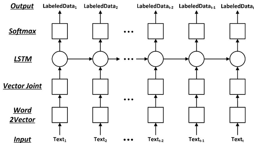
**Figure 4:** Schematic diagram of the LSTM model
