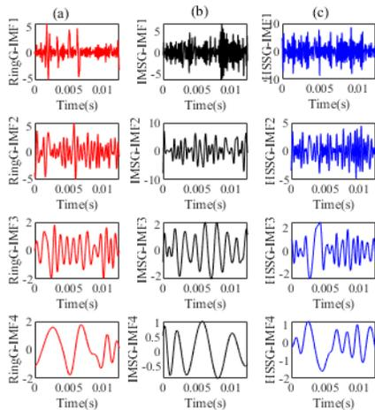
**Figure 6. Empirical Mode Decomposition (a) Ring Gear Vibration (b) IMS Gear Vibration (c) HSS Gear Vibration.**
