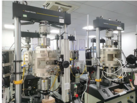
Figure 4: High temperature fatigue tensile testing machine (Instron 8801)
