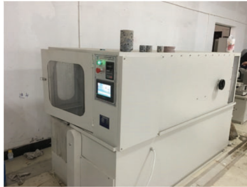
Figure 3: Self-developed rock and soil cutting and grinding machine
