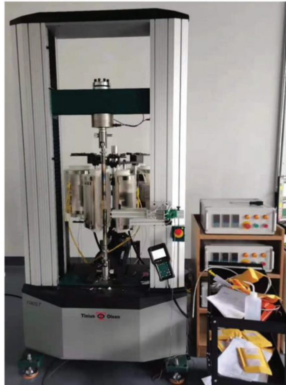
Figure 2: High temperature tensile testing machine (Tinius Olsen 100ST)
