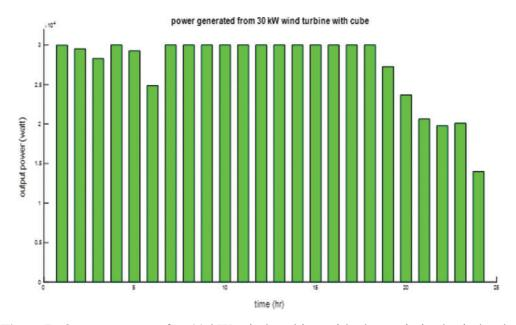
Figure 7: Output power of a 30-kW wind turbine with the optimized wind cube
