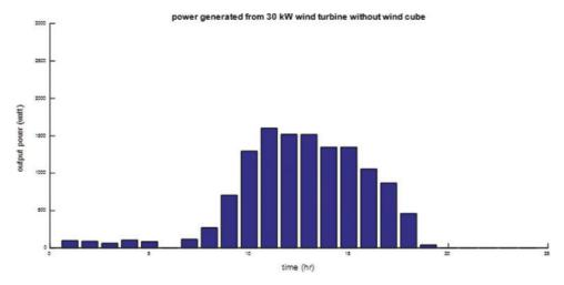
Figure 6: Power generated from 30-kW wind turbine without a wind cube
