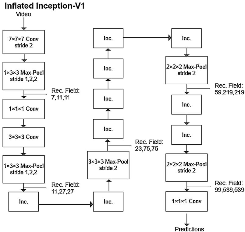
**Figure 3:** Network structure for I3D
