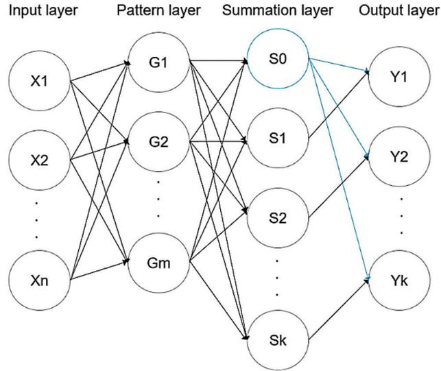
**Figure 4:** Network structure of a GRNN
