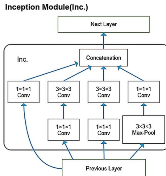
**Figure 2:** Network structure of an Inception module
