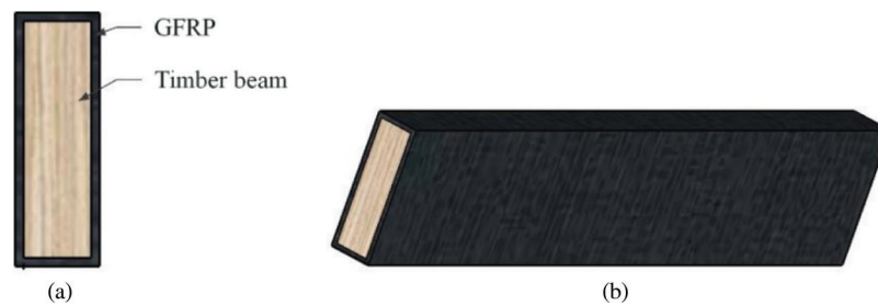
Figure 15: Reinforcement schematic diagram [91] (a is the sectional view, b is the longitudinal view)
